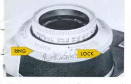
are using, then set this number on the camera as follows: Depress the selector ring LOCK and revolve the selector RING counterclockwise until the blue flash arrow snaplocks opposite the proper flash guide number on the lens mount (if impossible to set, change focus setting). A guide number of 70 is set in the illustration.
